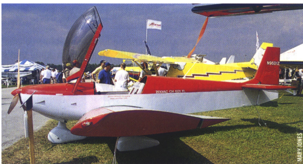
This profile shot of the Zenith Zodiac CH 601 XL gives a good view of the airfoil of the wing. The all-metal, two-seat, side-by-side aircraft meets the proposed light-sport aircraft parameters, making it a natural choice for sport pilots who like metal airplanes.
