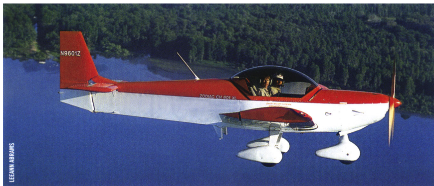
This profile shot of the Zenith Zodiac CH 601 XL gives a good view of the airfoil of the wing. The all-metal, two-seat, side-by-side aircraft meets the proposed light-sport aircraft parameters, making it a natural choice for sport pilots who like metal airplanes.
