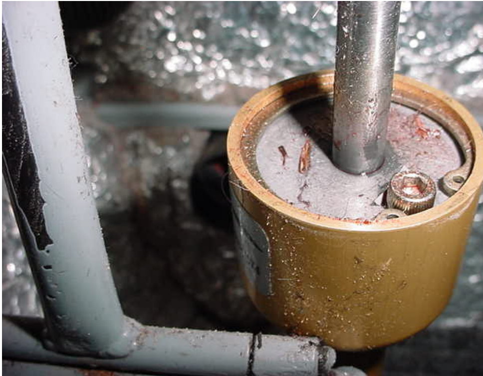
location of bleed screw at the bottom of the caliper (on one each wheel).
