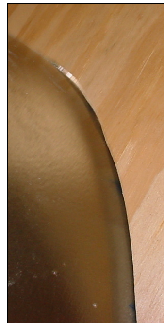
Look for the side that has minimum separate between the bubble and the plywood template.
