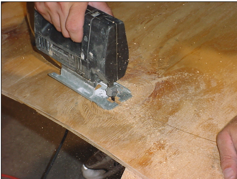
Use a jig saw to cut on the line. The critical part is the outside blank, if you have too cut small on the inside of the line, then go back and cut on the line.
